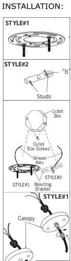
1. Refer to the mounting bracket style that matches the bracket that is included with your fixture.
